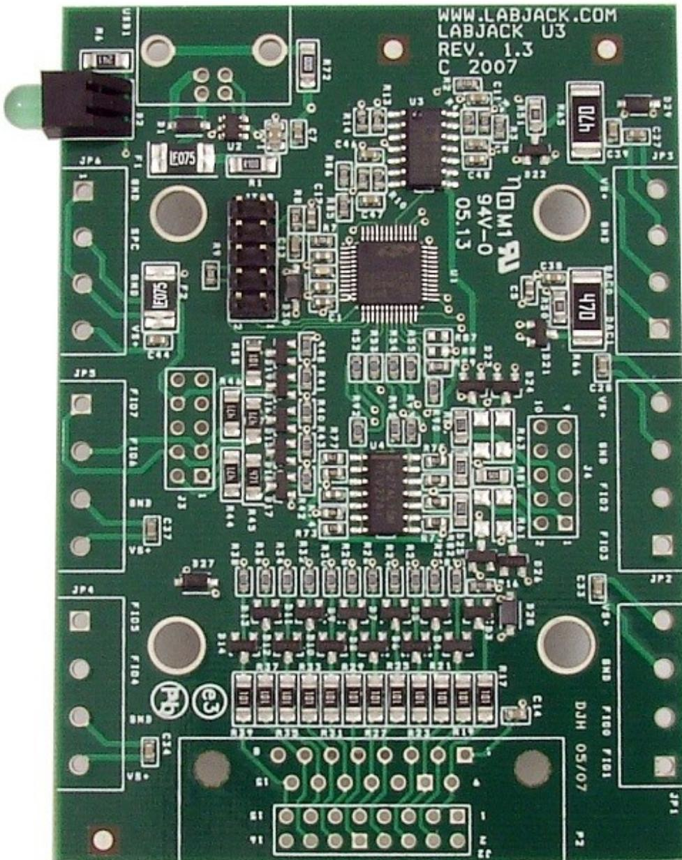
Screw-terminals are not installed. The PCB is designed for 5mm screw-terminals, but 5.08mm should fit also.
